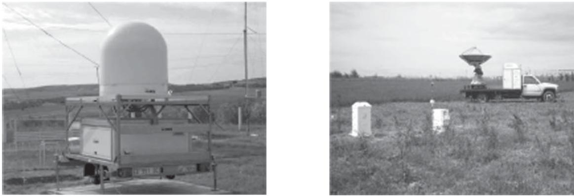
Fig. 2. One of the mini-radars (left) and the XPol mobile radar with the nearby disdrometer and gauges (right)
